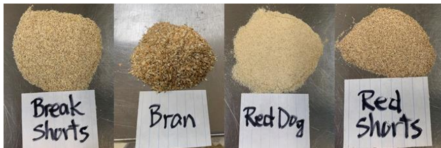
Figure 2. The mill produces the following offal streams, in order of mill output from left to right: break shorts, bran, red dog, and red shorts.
