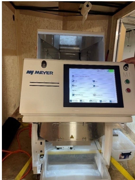
Figure 16. Meyer Color Sorter Adjusted for Cleaning Ergot and Small Black Weed Seeds from Kernza®
