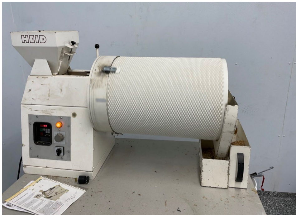
Figure 12. Lab Scale CIMBRIA Indent Separator with 7.9mm drum for in-hull/dehulled Kernza® separation
