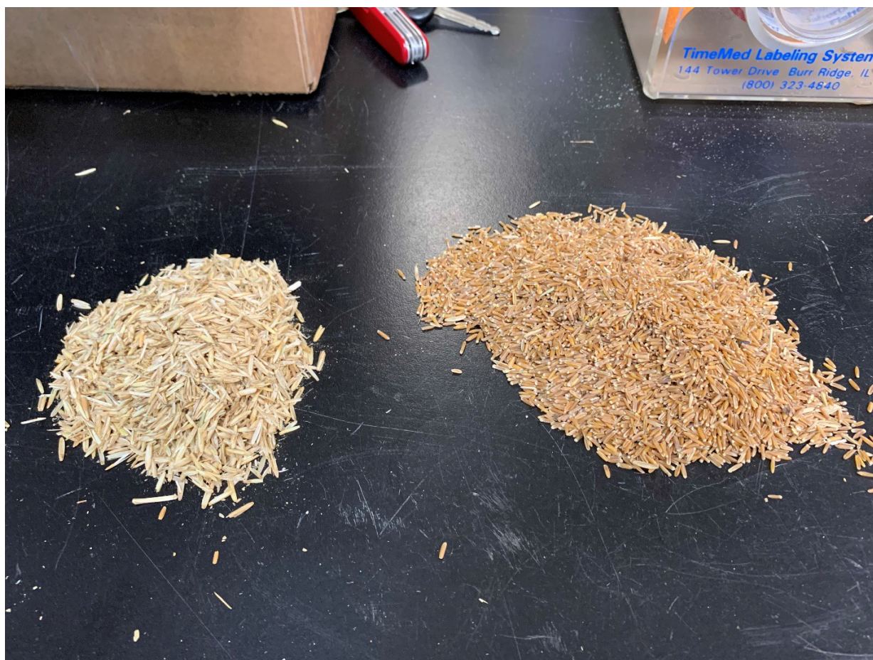
Figure 4: Separated Kernza® Grain and Hulls post dehulling on Model 15D Forsberg Huller
